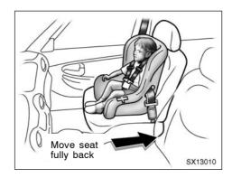
• A forward-facing child restraint system should be allowed to be installed on the front passenger seat only when it is unavoidable. Always move the seat as far back as possible, because the front passenger airbag could inflate with considerable speed and force. Otherwise, the child may be killed or seriously injured.
