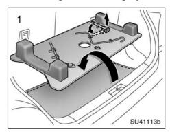
1. Remove and turn over the spare tire cover. Remove the front towing eyelet.
