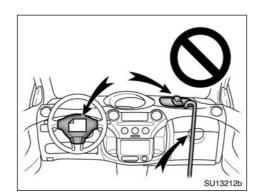
• Do not put anything or any part of your body on or in front of the dashboard or steering wheel pad that houses the airbag system. They might restrict inflation or cause death or serious injury as they are projected rearward by the force of deploying airbags. Likewise, the driver and front passenger should not hold objects in their arms or on their knees.
