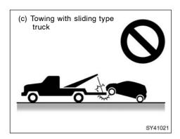
(c) Towing with sling type truck
