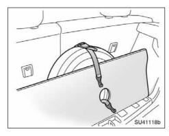
Put the spare tire cover against the flat tire, and then pass the rest of the belt hooks thorough the hole in the cover.
