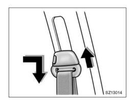
Seat belts with an adjustable shoulder anchor (5-door models)—
