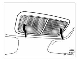
To turn on the personal light, push the lens. To turn the light off, push the lens once again.
