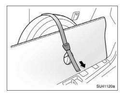
Hold the buckle and pull the belt. Securely tie the tire and spare tire cover.
