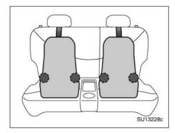
The lower anchorages for the child restraint system interfaced with the FMVSS225 or CMVSS210.2 specification are installed in the rear seat.
