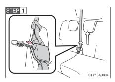
To release the hooked end tab, insert the vehicle's key into the hole on the buckle.
