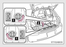
Turn the knobs to the UNLOCK position.
