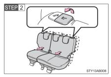
Pull the seat position adjustment lever up. Then slide the rear seat fully forward.
