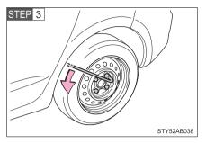
Slightly loosen the wheel nuts (one turn).
