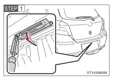
Disengage the claws and remove the license plate light.
