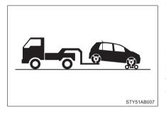
Vehicles with an automatic transmission: Use a towing dolly under the front wheels.
