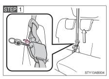
Insert the key into the hole on the center seat belt buckle to release tab (with hooked end), and allow the belt to retract.
