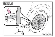
Vehicles with a steel wheel, remove the wheel ornament using the wrench.
