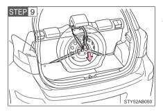
Hold the buckle and pull the belt to secure the tire.
