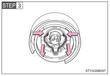
Release the bulb retaining spring.
