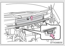
1.Push the tab in and lift the cover off.
