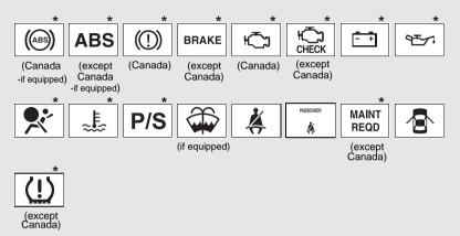
\*: These lights turn on when the engine switch is turned to the ON position to indicate that a system check is being performed. They will turn off after the engine is started, or after a few seconds. There may be a malfunction in a system if a light does not come on, or if the lights do not turn off. Have the vehicle inspected by your Toyota dealer.
