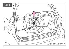
Pass the belt through the center hole of the flat tire wheel.
