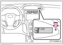
STEP 1 Press and hold the clock reset button to enter the adjustment mode for the clock.
