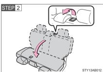
Pull the seatback angle adjustment lever up and fold the seatback down.
