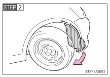
Partly remove the fender liner.
