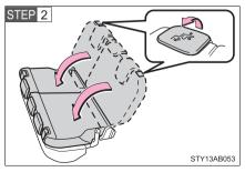
Pull the seatback angle adjustment lever up and fold the seatback down. n Folding down rear seatback (non-split rear seat)
