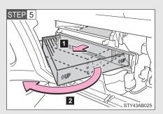
Pull out the filter.Rotate the filter to remove it.
