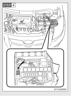
Remove the fuse with the pullout tool.
