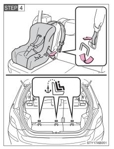
Latch the hook onto the anchor bracket and tighten the top tether strap.
