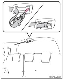
Stow the seat belt tabs in the cover set in the roof as shown.
