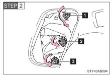
STEP 3 2 2 3 5 5TY43AB092 Turn the bulb base counterclockwise.
