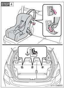
Latch the hook onto the anchor bracket and tighten the top tether strap.
