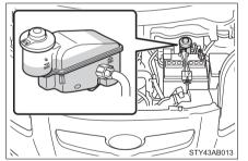
The brake fluid level should be between the MAX and MIN lines on the reservoir.
