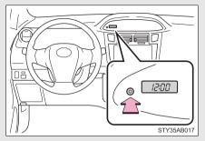
STEP 1 Press and hold the clock reset button to enter the adjustment mode for the clock.
