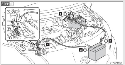
Connecting the jumper cables
