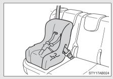
Seat belts equipped with a child restraint locking mechanism (ALR/ELR belts except driver's seat belt) ( $\rightarrow$ P. 52)
