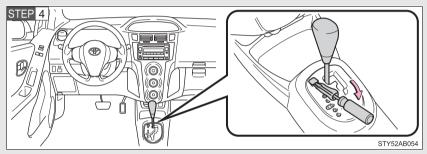
Pry the cover up with a flathead screwdriver or equivalent.
