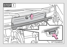
Push the tab in and lift the cover off.
