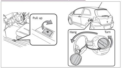
**NOTE:** Tighten until one click is heard. If the cap is not tightened enough, Check Engine "  $\bigcirc$  " indicator may illuminate.
