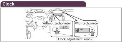
Press and hold clock reset button for adjustment mode. Press again to adjust minutes and hours, waiting 5 seconds after each.
